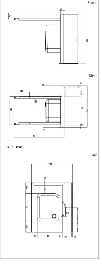
Handling System for Rack Type Pre-wash Table with Sink Left to Right, 900mm
